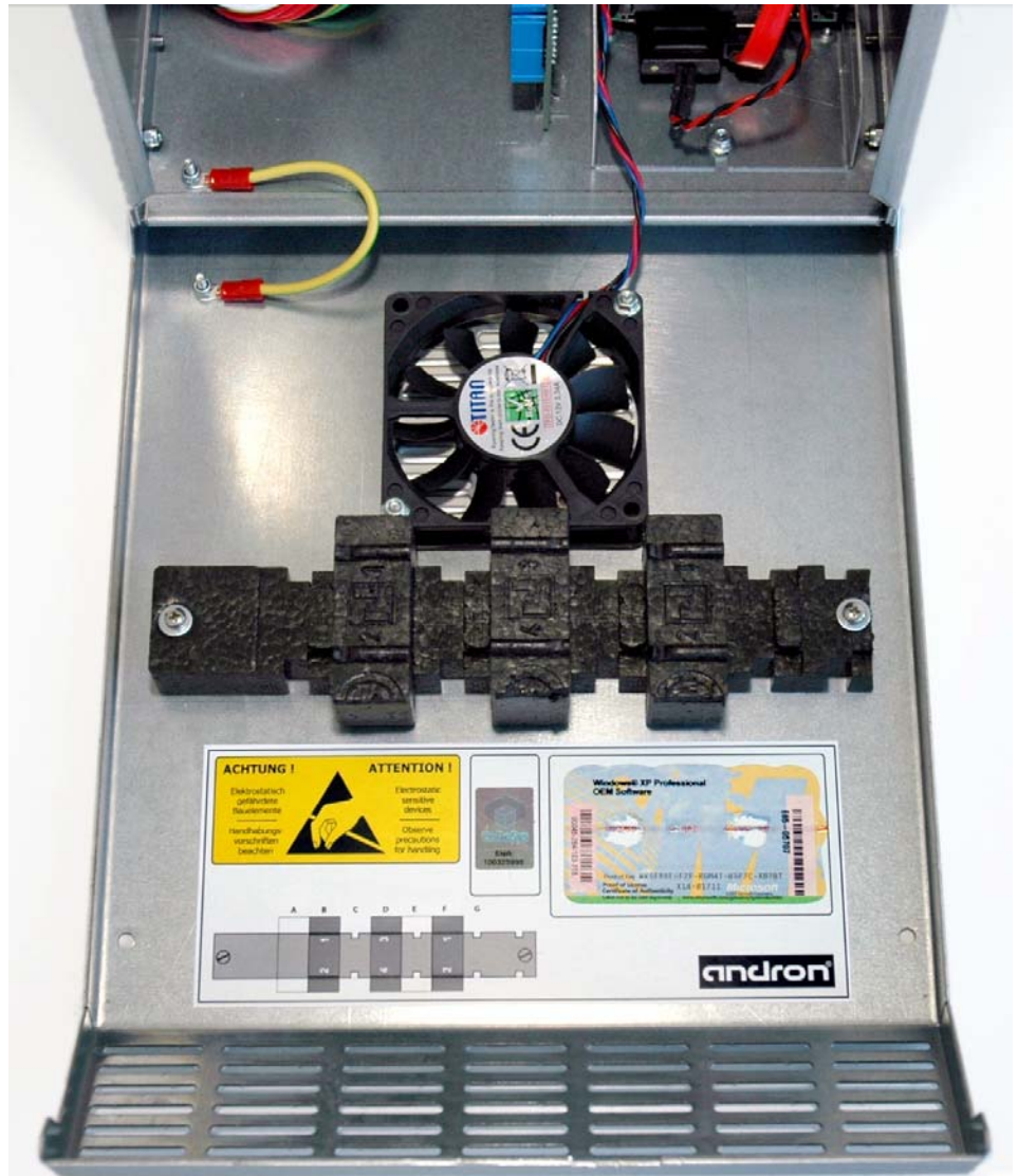
Illustration: Open control module with licence stickers, fans and card holder
