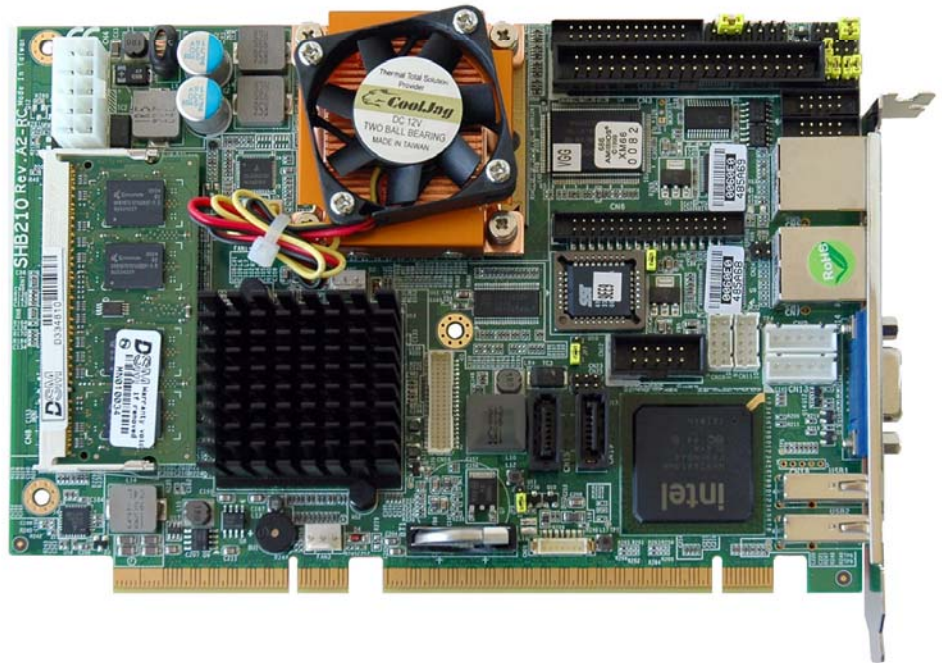
Illustration: Front side of the SHB210 with processor, all interfaces and DDR2 memory slot
